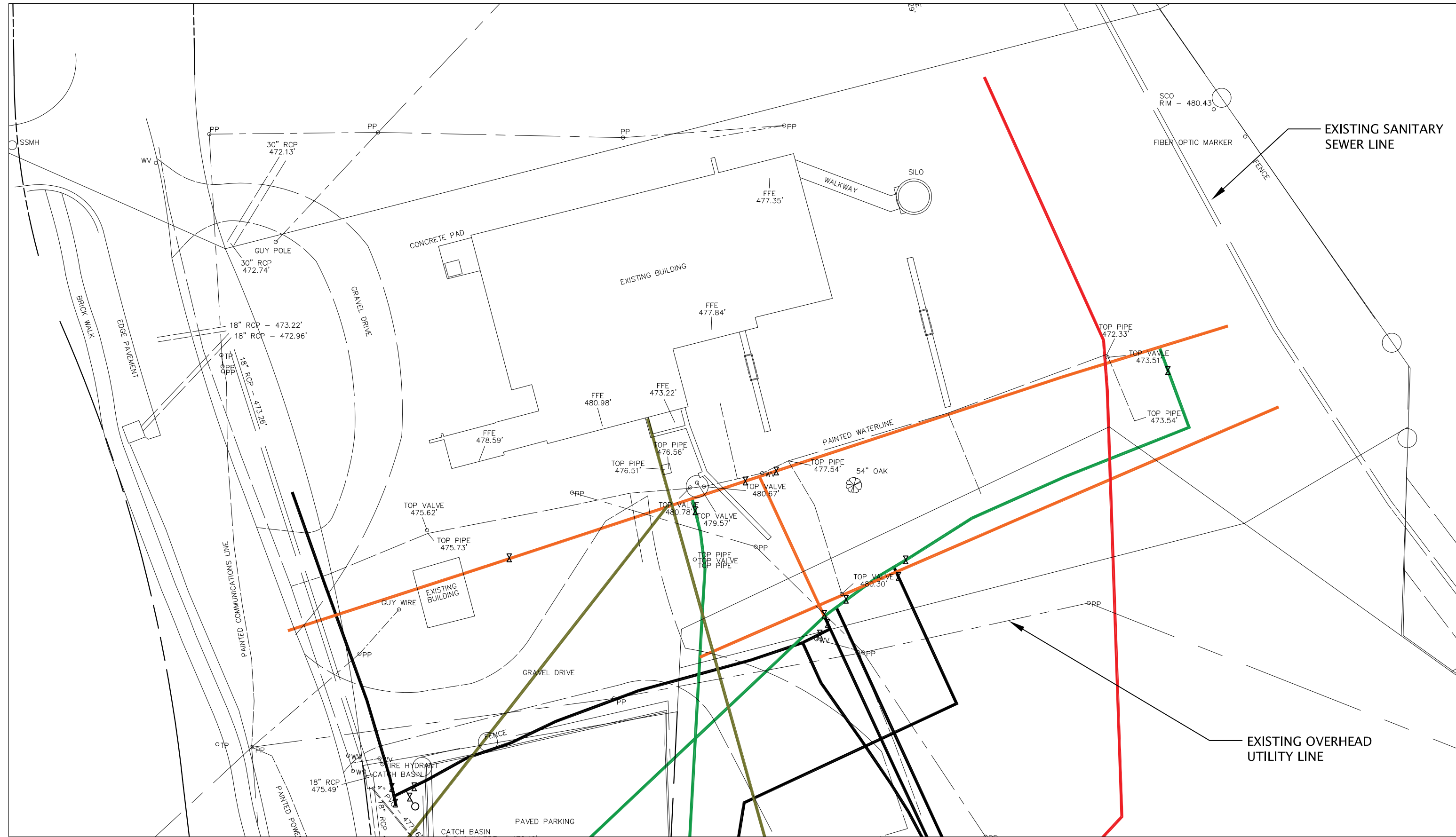
1 L2 EXISTING CONDITIONS & UTILITIES PLAN SCALE: 1"= 30'-0"
