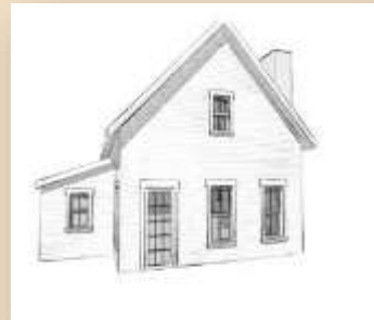
✓ A house with 6-inch casing on top of the window and 4-inch window casing on sides and bottom
