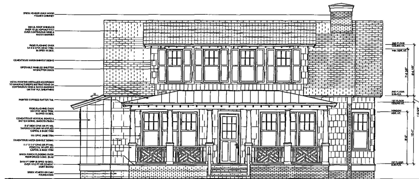
① FRONT ELEVATION SCALE: 1/4" = 1'-0"
