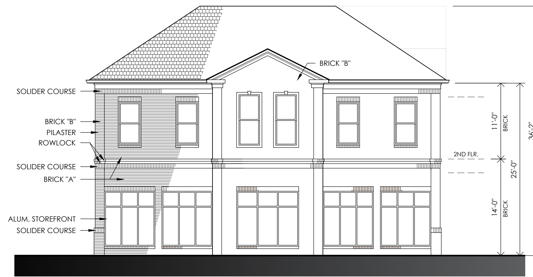
A1.1-02 NORTH BUILDING: E. ELEVATION
