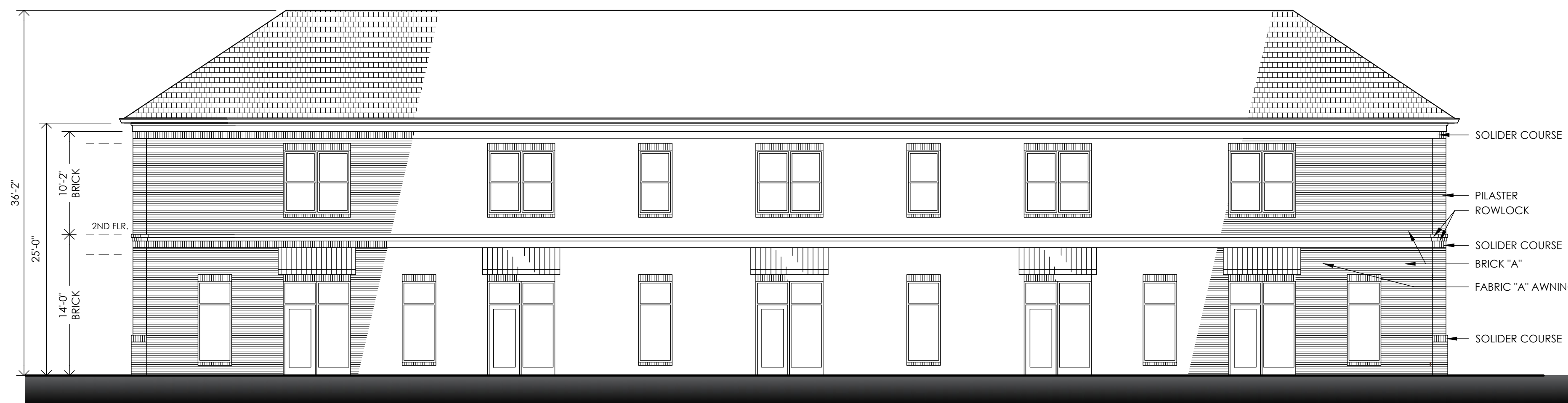
A1.1-03 NORTH BUILDING: S. ELEVATION
