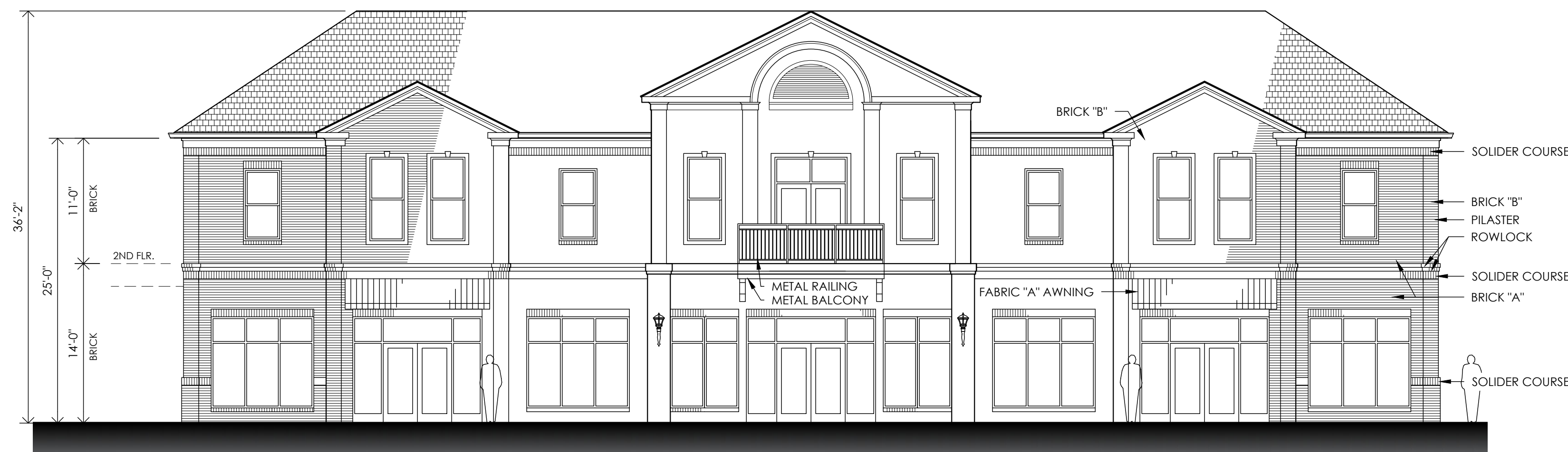
A1.1-05 SOUTH BUILDING: N. ELEVATION
