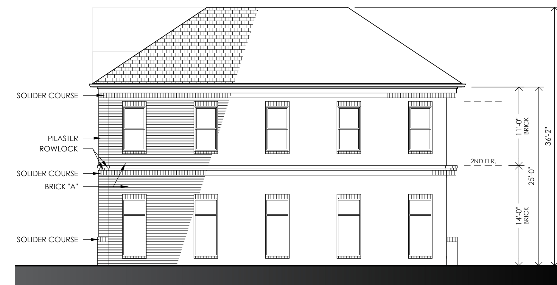
A1.1-04 NORTH BUILDING: W. ELEVATION
