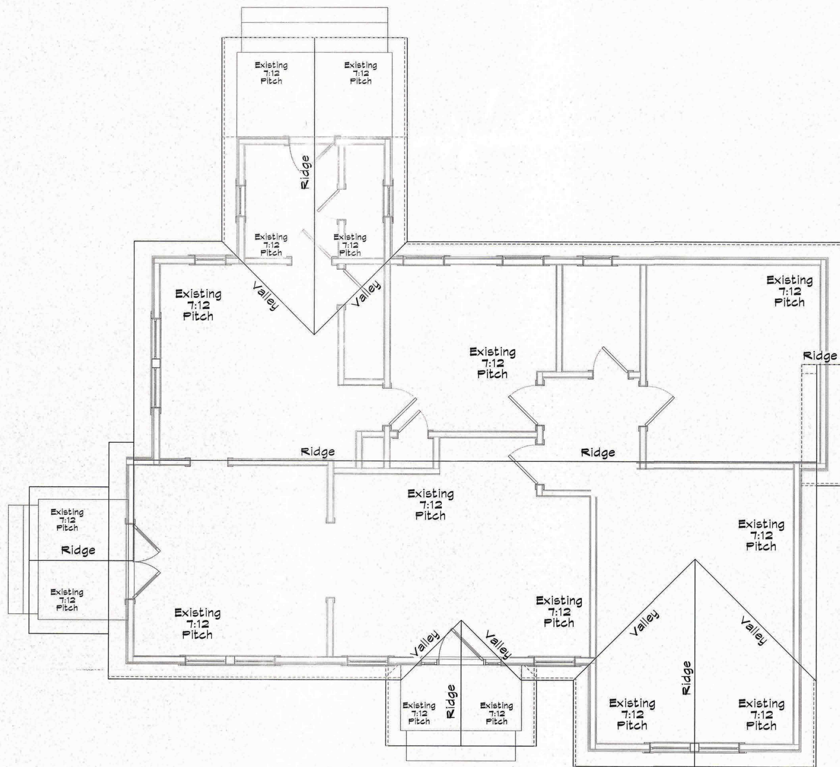
1 Existing Roof Plan Scale: 1/4" = 1'-0"
