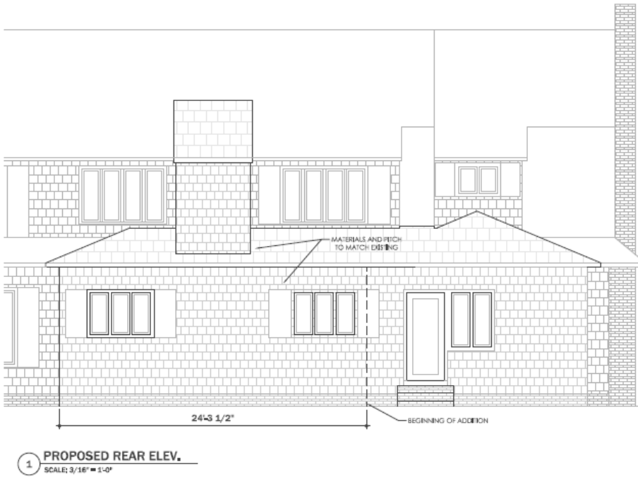
Proposed rear elevation (kitchen addition)
