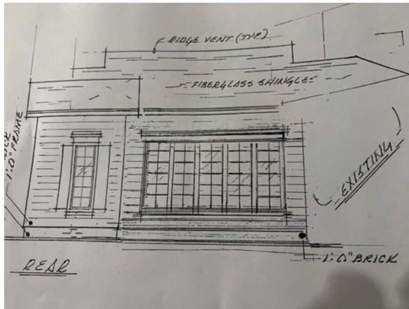
Addition windows showing (5) 7' windows next to existing.
