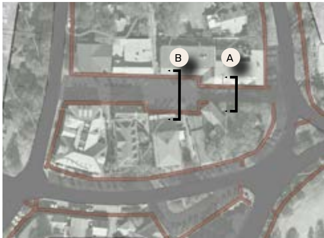
MARKET SQUARE TYPICAL SECTION (A) Market square near the Dogwood Road entrance provides a one-way drive aisle and parallel parking. A brick pedestrian walk accesses shops on the north side. A narrow vegetative buffer separates the drive aisle and the building to the south.
