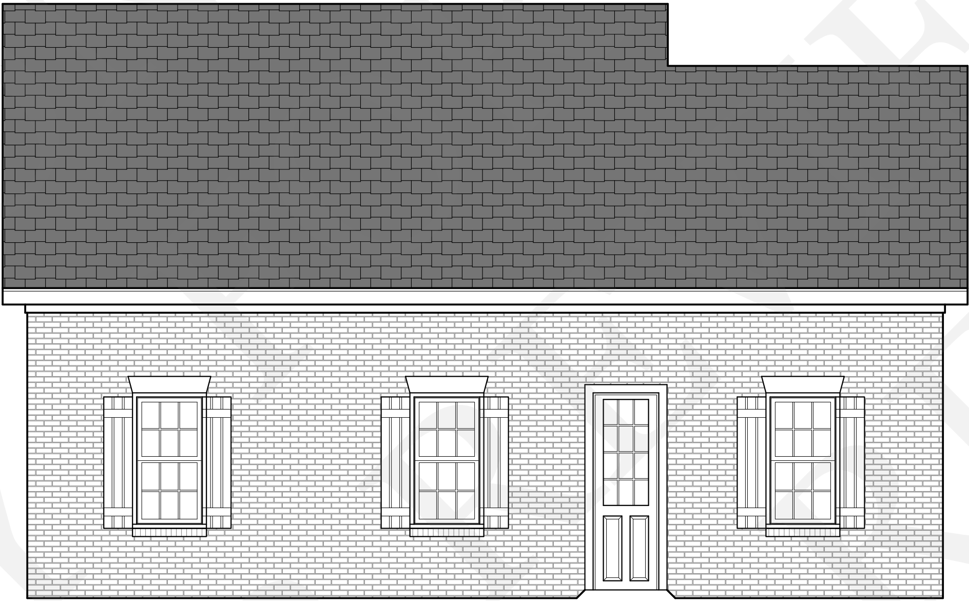
DETACHED GARAGE LEFT ELEVATION 1/4" = 1'-0"
